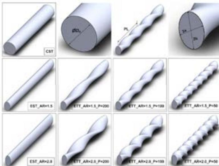
**Figure 1.** Considered tube configurations in the study
