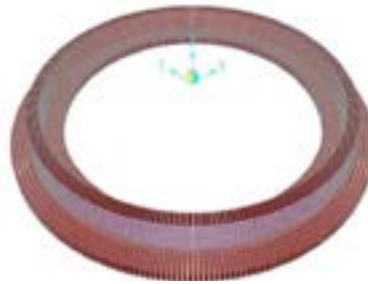
Figure 8: Ring wall foundation design
